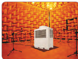
Noise testing lab
